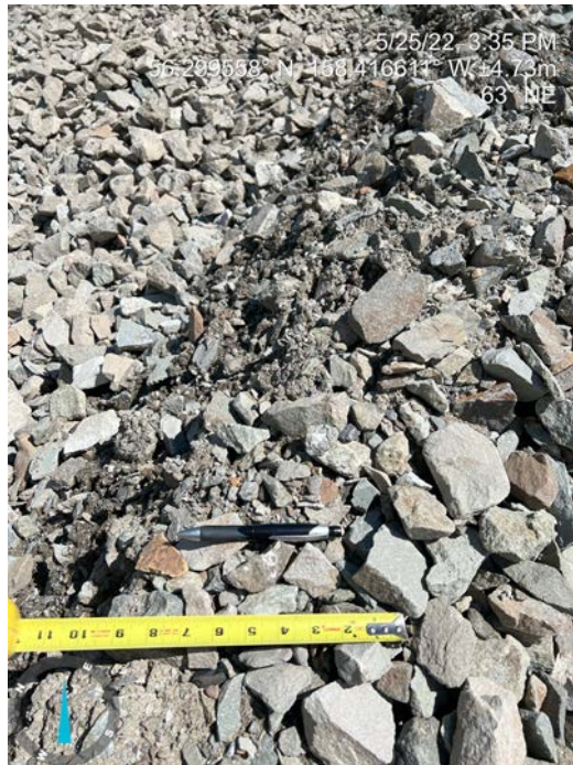
Rock Pile Gradation
