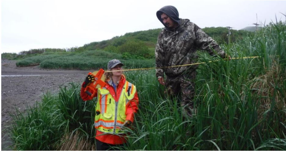
Figure 2. Example of measuring from a stake to an eroding bluff at Chignik Bay, AK.
