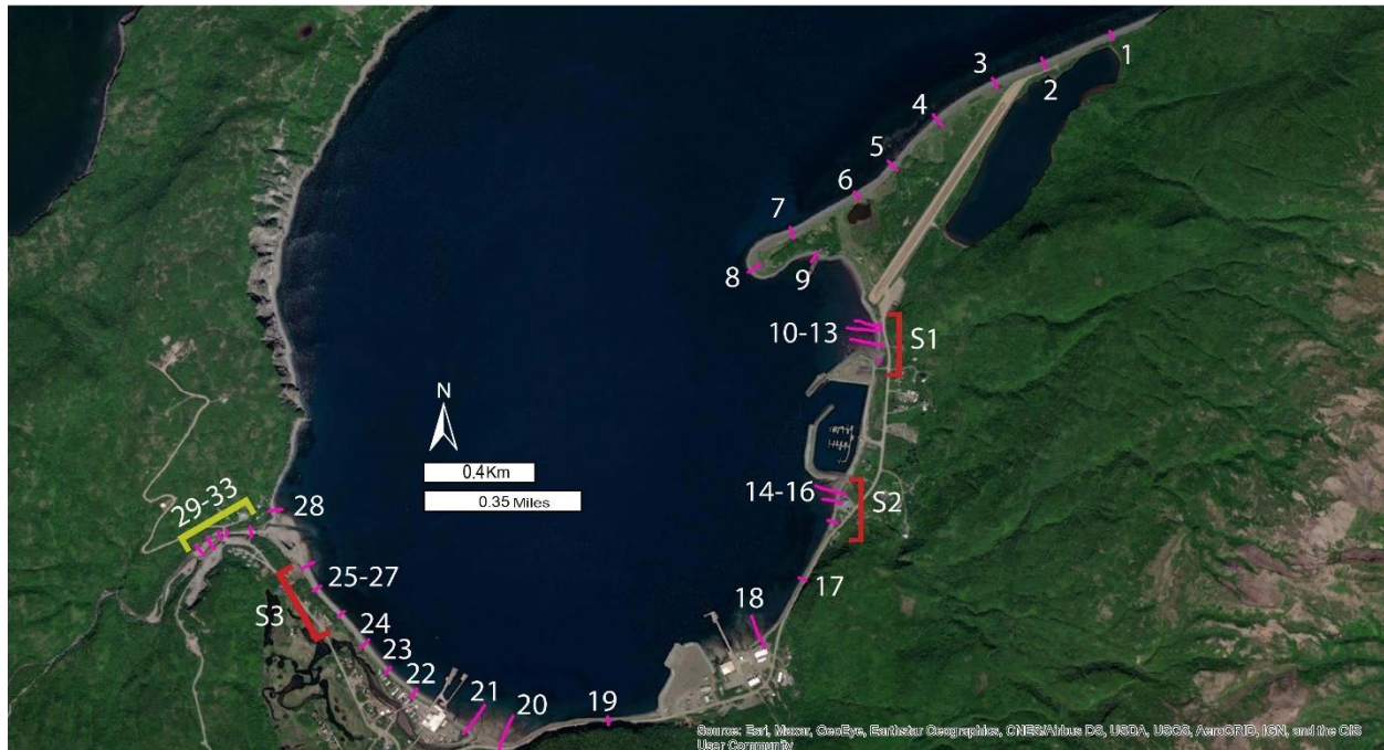
Figure 24. Map showing the location of each cross-shore elevation profile. Red brackets represent CBM sites. Yellow bracket represents cross-river elevation profiles.
