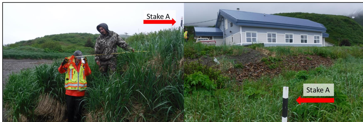
Figure 2.6 (Left) Chignik Bay environmental observer (Ed Krauss) and ACGL student (Jessie Christian) collecting stake ranging measurements at the Chignik Bay medical clinic erosion monitoring site. (Right) Stake A at transect 1, positioned in front of the Clinic on unconsolidated sediment.
